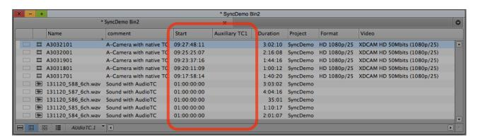
Here is a typical example of how to use Audio-Timecode for syncing. In this example we have video of a Canon C300 camera wich has native timecode. The audio comes from a Tascam DR680 wich is a 6 channel audio recorder without native timecode capabilities. Here timecode has been recorded as an audio signal onto one audio track (which sounds like a strange noise).
