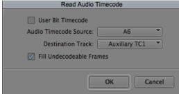
To extract Audio-Timecode of clips and convert it into a native timecode track you just have to select the respective clips and use the "Read Audio Timecode" function of the "Special" menu. A window will open where you are able to select the following settings:
